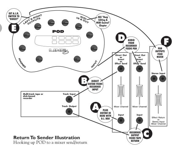
Plug the guitar into your DI. Plug the DI into a mixer channel with a direct out. Set the trim on your channel so your input levels look good. Plug the direct output from the mixer channel into one of your recorder's track inputs, and set the recorder to monitor the input to that track. Connect the recorder's track output to another mixer channel input that has a direct output. Plug that direct output into your POD's input, and plug the POD outputs into one of your mixer's stereo
